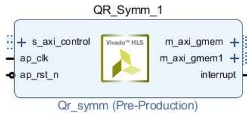
Figure 3.2.2 IP of QR Algorithm in Vivado Design Suite
